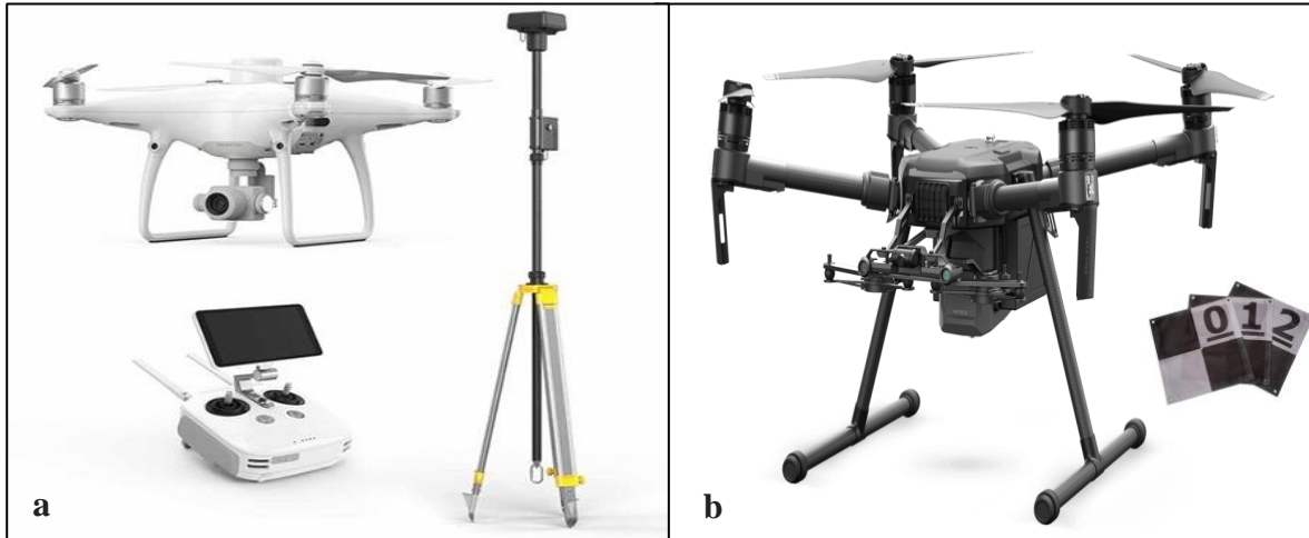
Drone platforms used for the pilot project: the DJI Phantom 4 Pro+ RTK with corresponding base station (a) and the DJI Matrice 210 with Ground Control Points (b).
