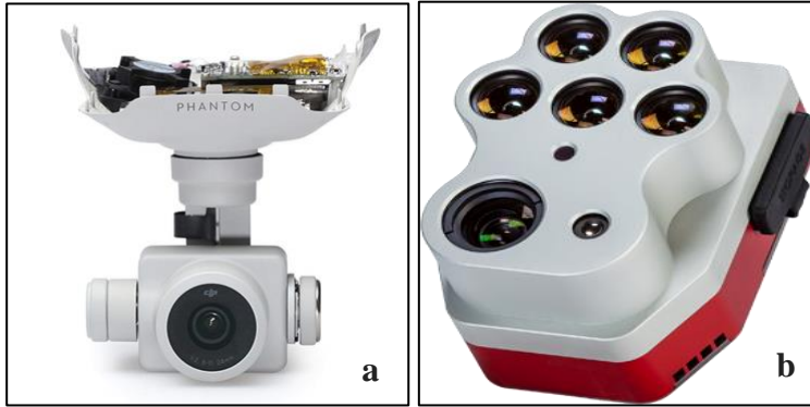
Drone sensors used for the pilot project: the Phantom’s RGB optical camera (a) and a Micasense Altum multispectral sensor (b).
