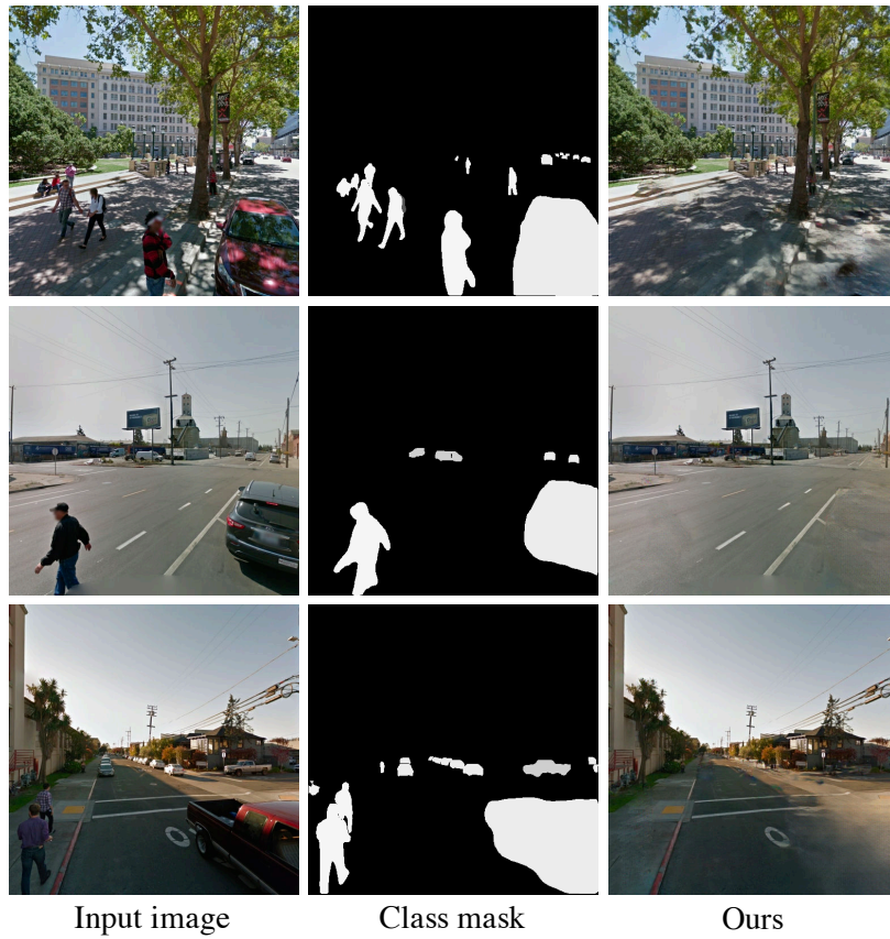
Figure 3.12: Qualitative results for removing all people and cars in a street image. From left to right: the input image, the class mask for objects to be removed, and the removal results generated by the removal network. Our method removes objects completely.
