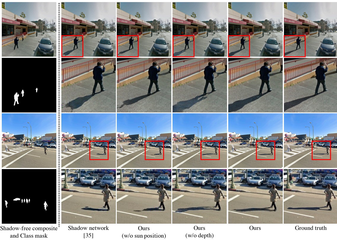
Figure 3.11: Object insertion results on the test set. Our method generates the most realistic shadows with details. The sun position input helps the network to determine the shape of the shadow. The depth map prevents the network from synthesizing broken or detached shadows.
