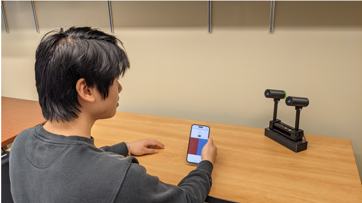
Figure 6.1: A prototype “two-headed” form factor that enables Beacon to present two different light stimuli simultaneously.
