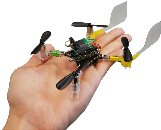
Figure 1.1: The Smellicopter is a modified commercial Crazyflie drone with custom electroantennogram circuit and wind fins for passive upwind orientation.
