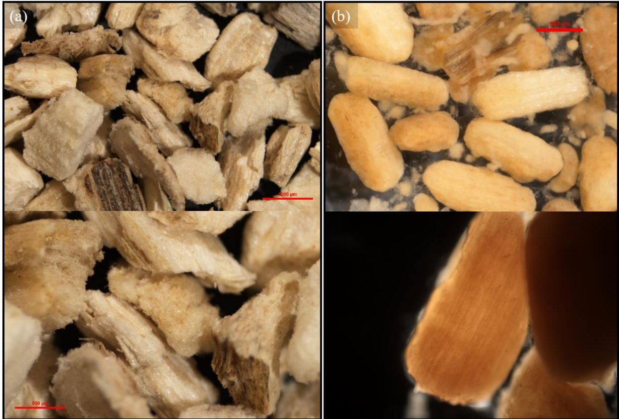
Fig. S3. (a) Dry kenaf media without biofilm growth; (b) kenaf granules after almost 2 years of biofilm buildup.
