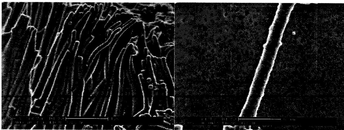
Figure 4-2 SEM micrographs of Au-coated SiO 2 nanorods. Left, 100 nm SiO 2 with 22 nm of Au. Right, 100 nm SiO 2 with 24 nm of Au.
