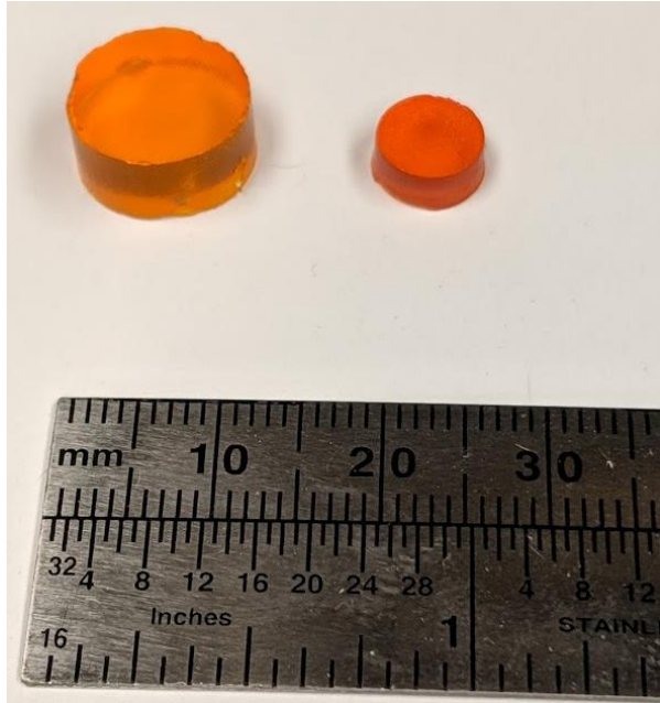
Figure B. 3 Printed compression disk at equilibrium swelling (left) and dehydrated (right). Formulation: 30 wt% MA-BSA with 5 wt% PEG-DA.
