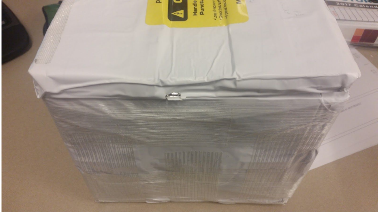
Figure 17 - Example of a tear in the Credo cooler’s VIP.
