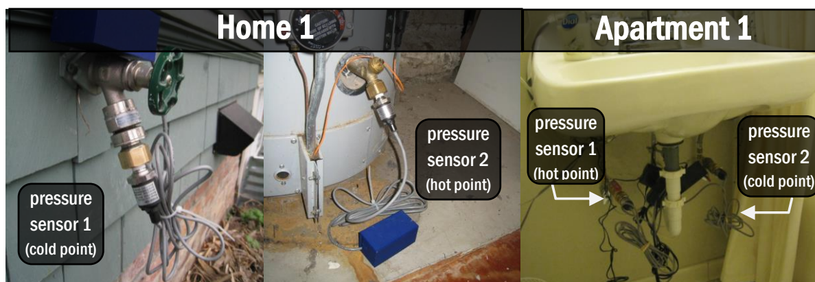
Figure 5-3. Two pressure sensors were installed at each deployment site (one on a hot water access point, one on a cold) in order to study the effect of installation points on classification accuracies.
