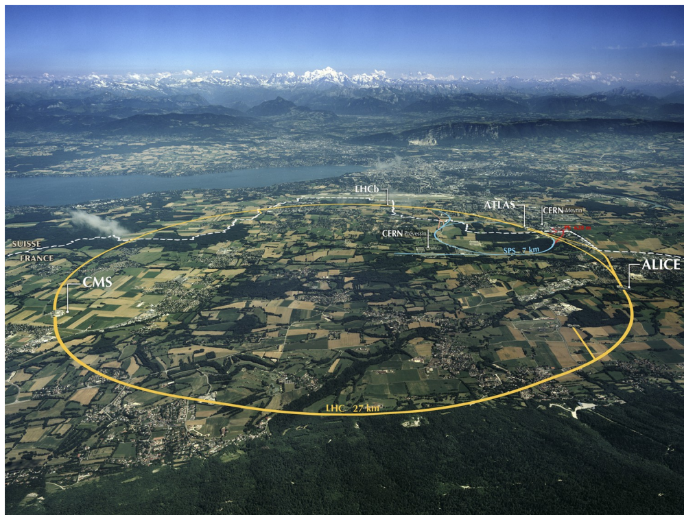
Figure 1.2: Aerial view of the LHC and its associated experiments [2]. The LHC is the world's most powerful particle accelerator in operation, capable of accelerating bunches of protons along a 27 km ring to an energy of 6.5 TeV each. At this energy, protons travel around the ring 11245 times per second. Each bunch contains roughly 100 billion protons. Bunches travelling in opposite directions around the ring are intentionally collided at experiment locations, resulting in approximately 1 billion proton-proton collisions per second [3].
