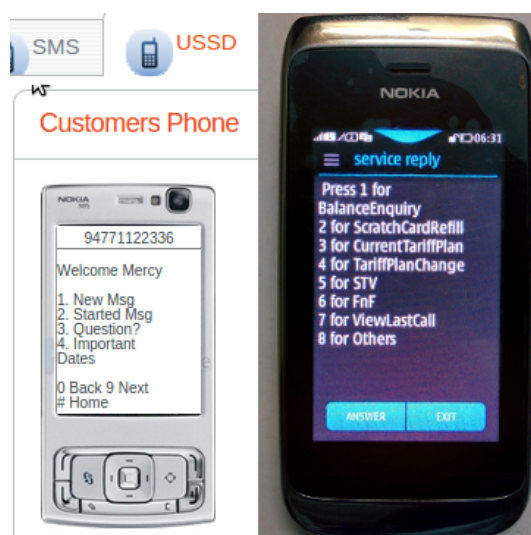
Figure 7.2: Left: Example Maternal Health USSD application running on IdeaMart USSD Simulator; Right: USSD home screen for Indian mobile operator BSNL.
