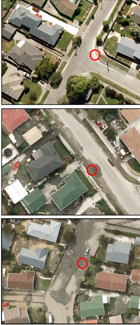
Figure 1. Representative observations of three classes of manifestation severity: (a) marginal; (b) moderate; and (c) severe, in accordance with the Green et al. (2014) criteria.
