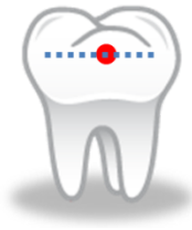
Figure 34: Protocol for obtaining dual laser fluorescence from a tooth. The red circle indicates a suspicious region to be measured. AF spectra are obtained at intervals of approximately 2 mm along the dashed line which spans through both sound enamel and the suspected carious lesion. The baseline reading is taken to be in a sound enamel region furthest away from the lesion and the lesion measurement is taken to be the centermost reading within the lesion area.
