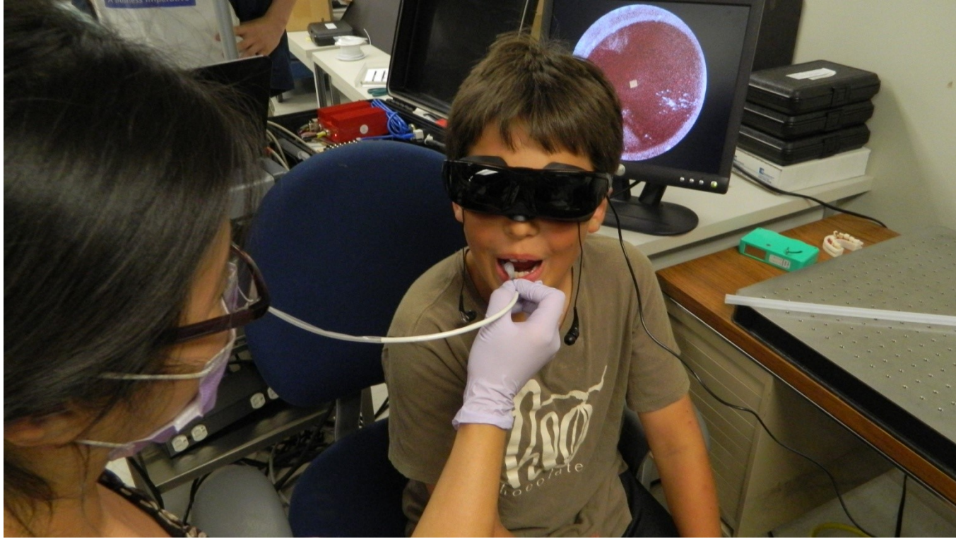
Figure 33: Use of the prototype device in vivo. The small size and flexibility of the fiber optic based probe is ideally suited for use in children. Note the display of the video image in the background. The image displayed on the screen is of the patient’s tongue.
