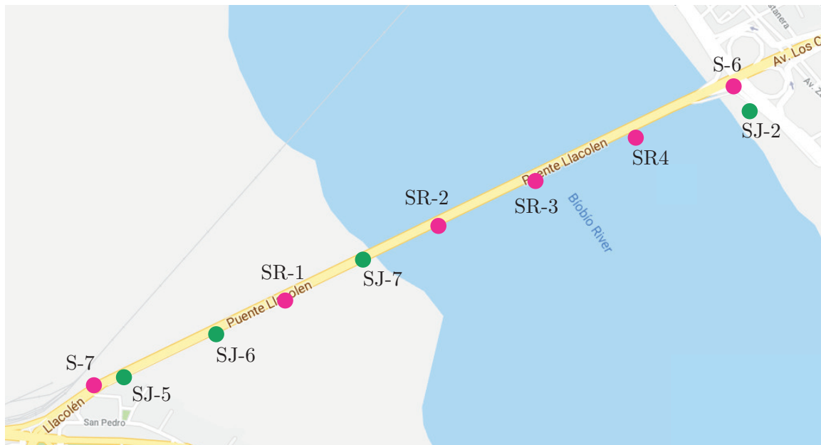
Figure 3.9: Location of Standard Penetration Tests along the bridge axis. Picture taken from www.maps.google.com .
