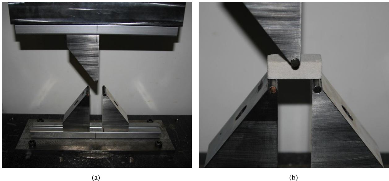
Figure 8. Experimental setup for 3-point bending test. (a) Test fixture (b) Flexure specimen positioned in fixture.
