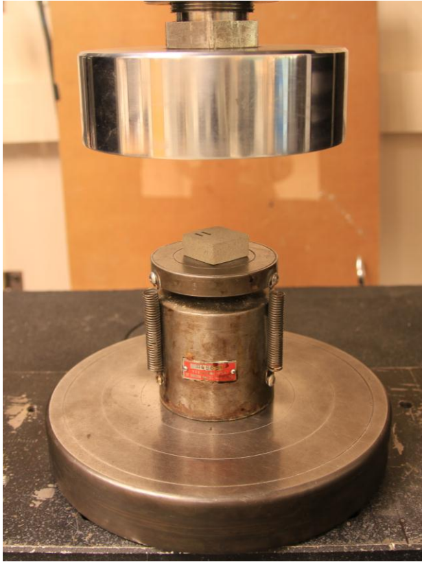
Figure 7. INSTRON 5585H outfitted with spherically seated bottom bearing plate.
