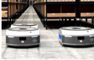
(c) Warehouse robots avoiding each other to retrieve packages.
