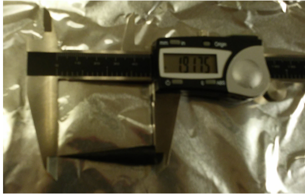
Figure 2.15: The cone shaped terminator manufactured for the second phase of the experiment. A mixture of epoxy and graphite is used to cast the terminator.
