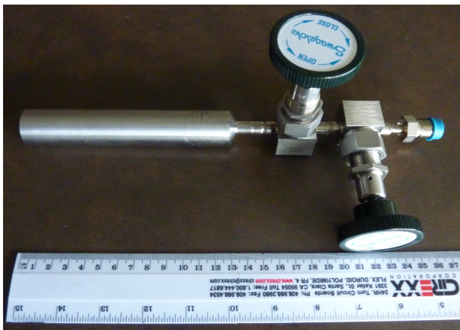
Figure 2.22: The cylinder built for storing 2Ci of tritium. The VCR valves are welded to the cylinder for safety reasons. They also facilitate a controlled release of tritium into the gas system.
