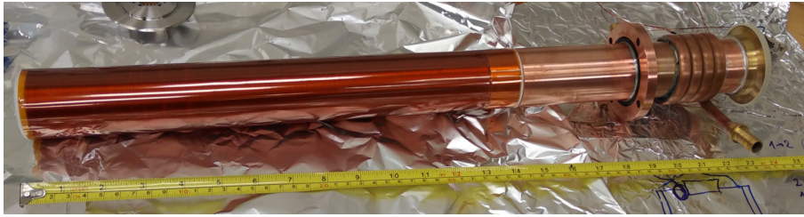
Figure 2.19: The field shifting solenoid designed to change the background field, and hence the cyclotron frequency of mono-energetic electrons from ^{83m}\text{Kr} . This coil is used in the study of frequency-dependent systematic effects introduced by the complicated receiver chain. The pipes are welded to the solenoid to cool it down during high current runs.
