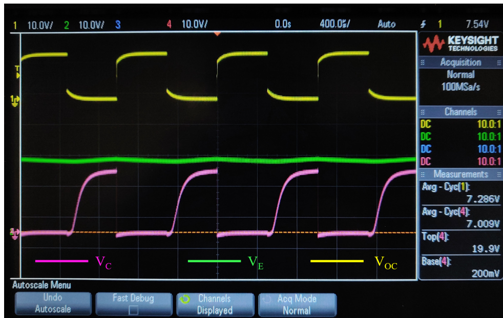
Figure 3.3: Three waveforms show the switching performance of our low-side switching circuit for a low voltage (22 V) test case.
