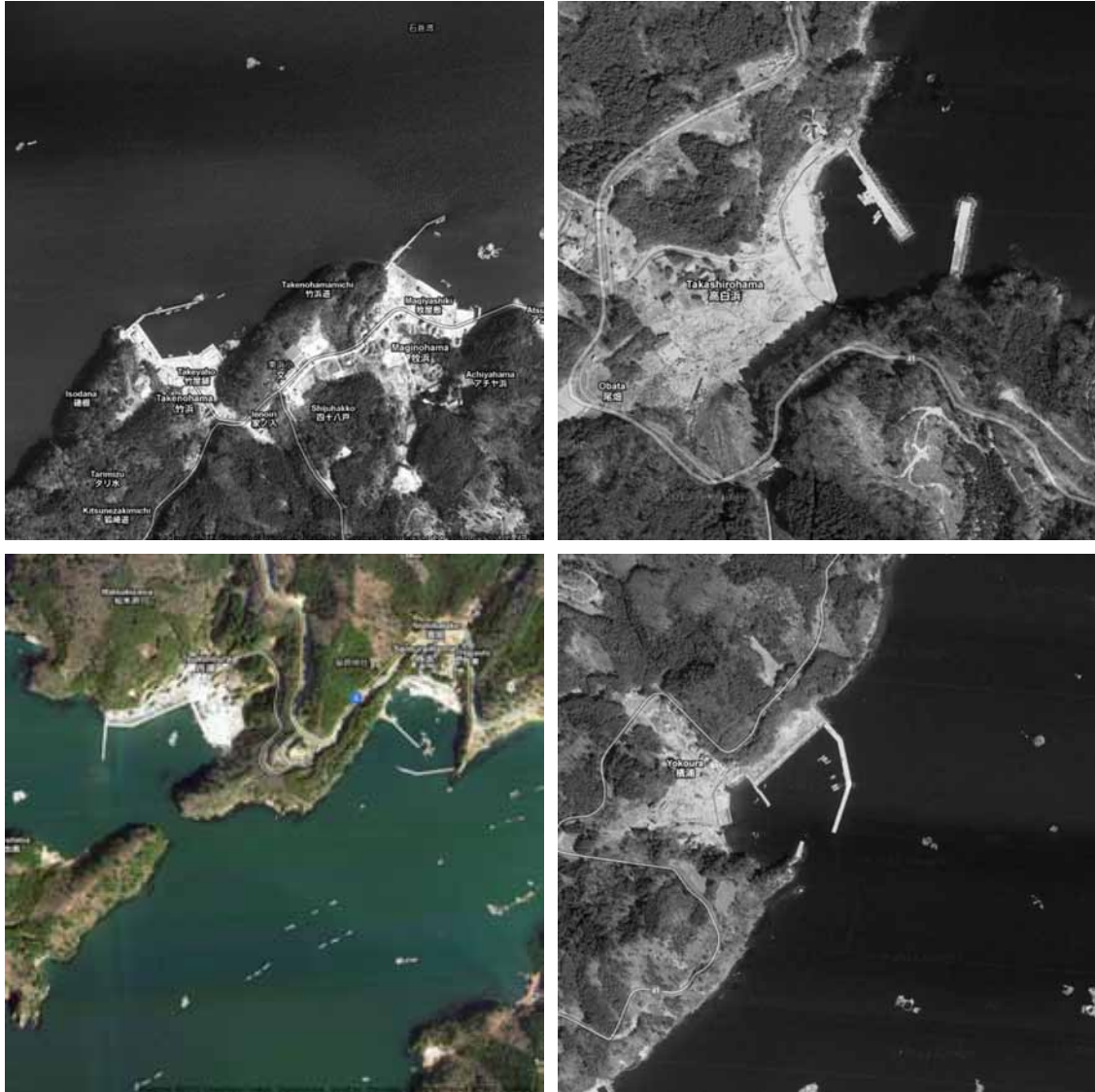
Figure 3. The fishing villages on the Oshika peninsula bear the unique marks of periodic tsunami: each has a seawall built perpendicular to the dominate current, an access road built to the level of the highest waterline on record (which would have swept away the former road). Careful inspection reveals remnant cedar farms on the hillsides, small agricultural fields, a few hillside shrines, and one or two well constructed concrete structures that doubles as an emergency shelter. From upper left, Tsukinoura/Samuraihama village, Takashirohama village; Takenohama/Maginohama village; and Yokoura village.
