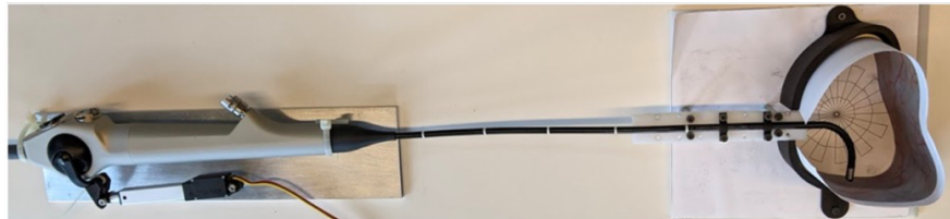
Figure 2.19: Test fixture for robotic cystoscopy data collection with Actuonix linear servo driving tip-bending lever. The 2.5D printed model approximates surface curves that may be seen in cystoscopies.
