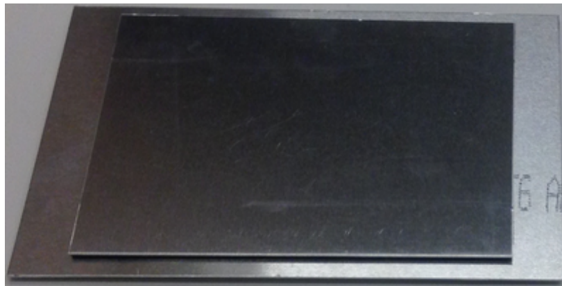
Figure 4.6: Bare electrode, a “guidance plate” without any holes.
