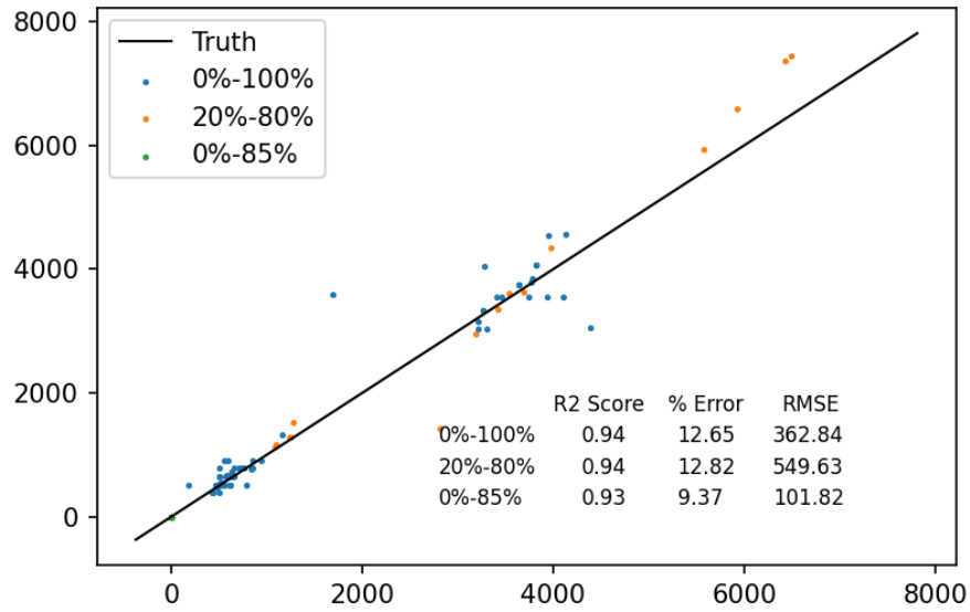
Figure 39. Performance metrics of the neural network with respect to different depths of discharge.
