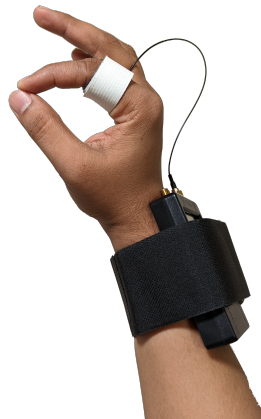
(b) A user wearing the Z-Ring prototype with a portable VNA strapped to their wrist.
