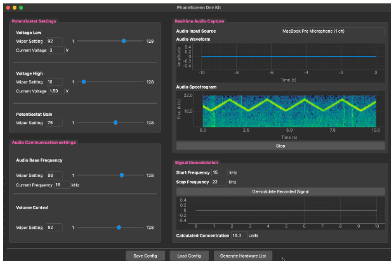
Figure 4.3: The PhoneScreen Companion Software interface, displaying real-time potentiostat settings, audio input visualization (waveform and spectrogram), and signal demodulation results, including calculated concentration.
