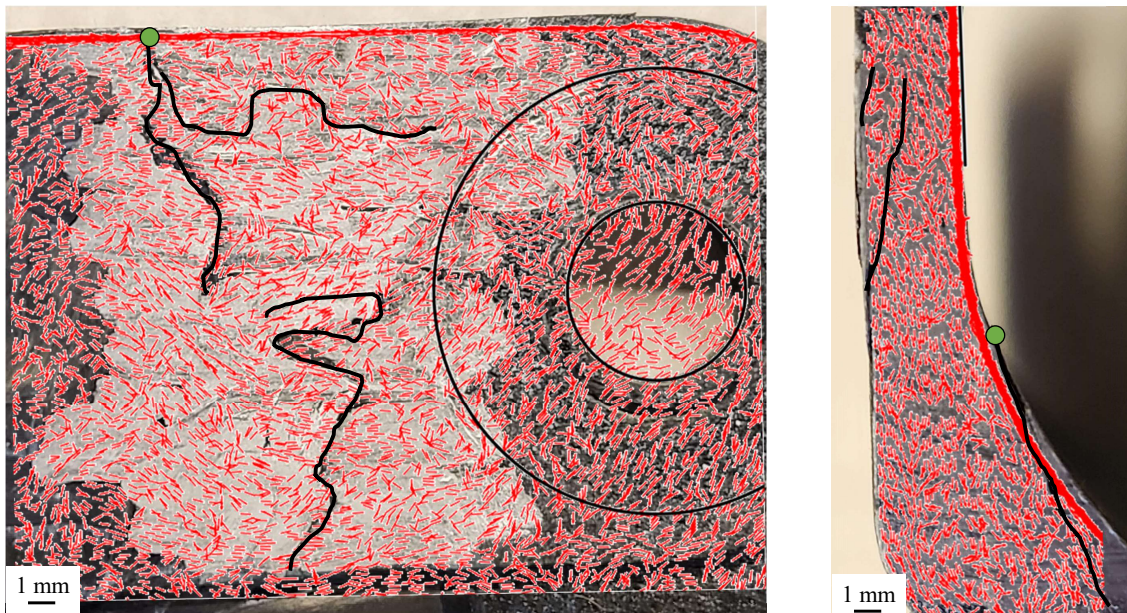
Figure A.6: Vector plots of narrow platelet Sekisui brackets of the orientation with the fracture path in bending.
