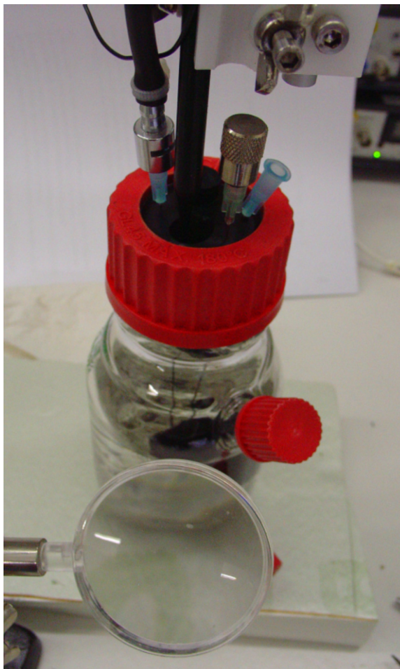
Figure B.1: Experimental setup, showing the mat-containing anaerobic incubation chamber, sulfide microsensor, and gas-exchange lines.
