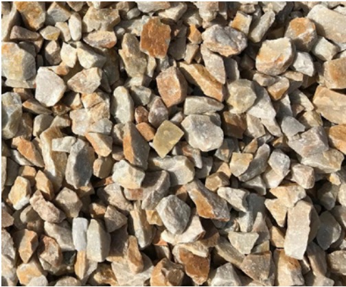
Figure 6.8: Gravel aggregate. (Vigoro)
