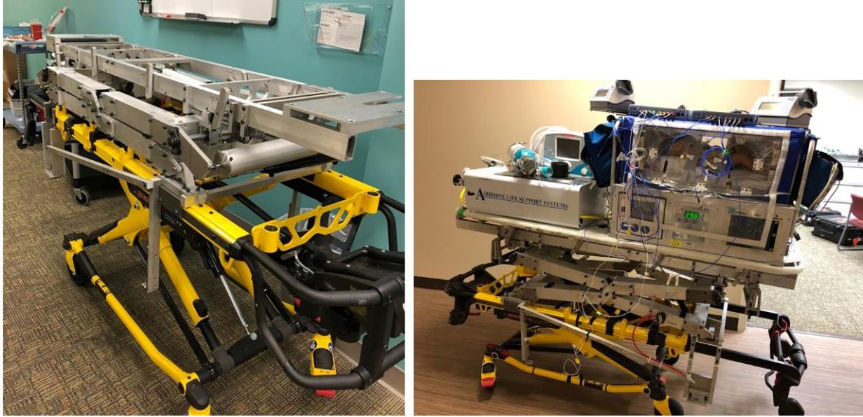
Figure 3.4. New stretcher system with the built-in suspension (left) and with the transfer sled and isolette (right)
