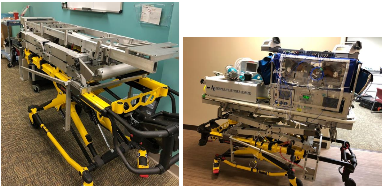
Figure 4.4. New stretcher system with the built-in suspension (left) and with the transfer sled and isolette (right)
