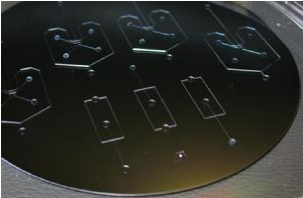
Figure 5: Patterns created on a master mold (Si wafer) using photolithography 13
