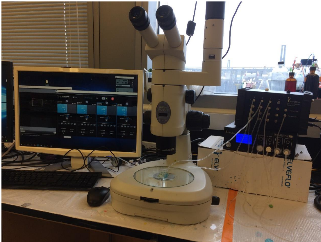
Figure 49: The interface of the air pressure control system- Elveflow. OB1 MK3, which is a pressure supply, provides positive and negative pressures ( \pm 14 psi) to control microfluidic flow systems. MUX, which is a microfluidic flow switch matrix, can be connected to OB1 MK3 and provides up to 16 pneumatic channels with controllable on/off sequences.
