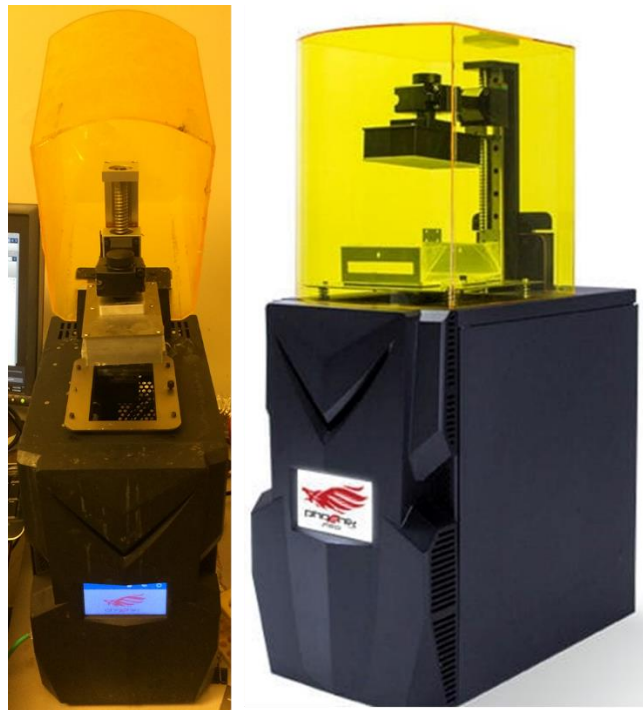
Figure 26: Photograph of Phoenix Touch Pro Translating UV-LED DLP 3D Printer. 40
