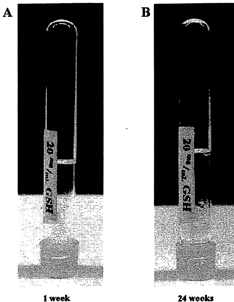
Figure 4.2: Photographs of 'fresh' and 'aged' gel prepared at 20 mg/mL GSH in DMSO. 4.2 A, after 1 week the gel appears completely transparent; the tube is inverted for the photograph to demonstrate the rigidity of the gel. 4.2 B, after 24 weeks, numerous small pockets of semi-transparency have appeared giving the gel a partly cloudy appearance; integrity of the gel, however, is not compromised.
