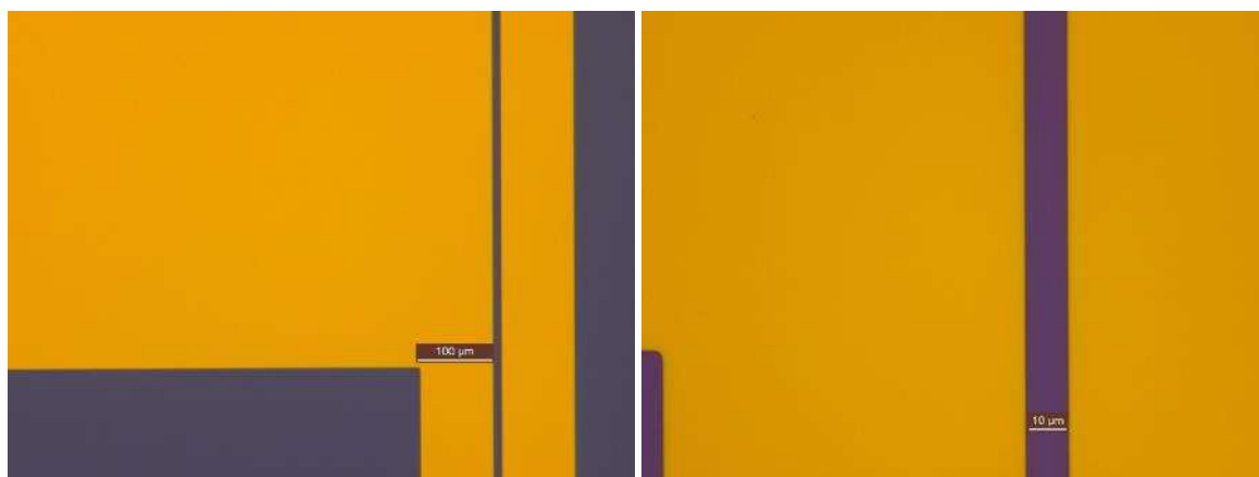
Figure 3.8 Microscope images of the insulated interdigitated back contact substrates used to determine the impact of electric field only on phase segregation of a MAPb(I 0.6 Br 0.4 ) 3 film. (Left) A 10x magnification image of one of the gold contact pads shown in the top left portion of the image and a 10 \mu\text{m} channel spanning from the top to bottom of the image. (Right) a 50x magnification image of the 10 \mu\text{m} channel.
