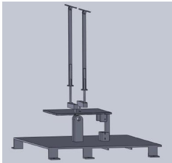
Figure 2.12. Example of design of 3-component force balance by Tintoré [45].
