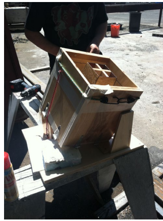
8. tilted mold assembly
