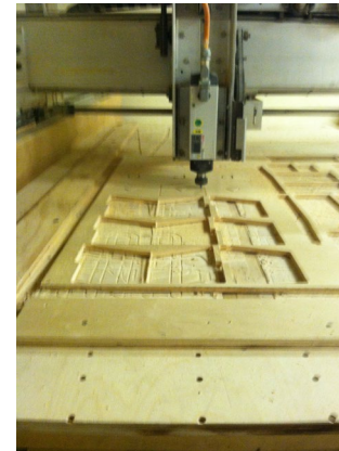
1. angular profiles being cut
