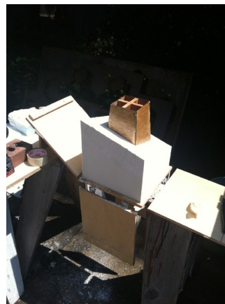
13. cast ready // curing time : 1 day
