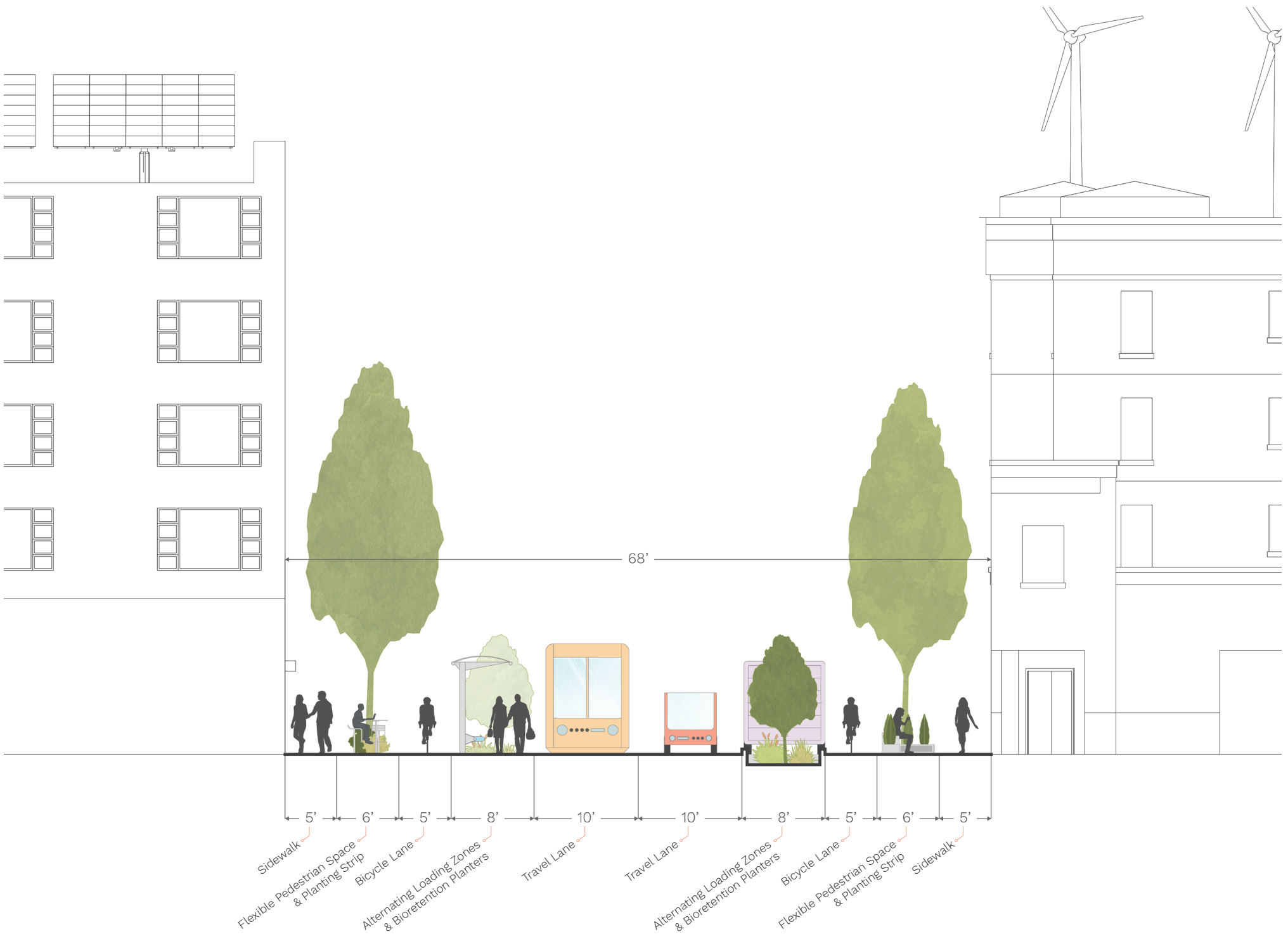
Figure 4.43: E Madison Street Design Proposal Section (Facing East)
