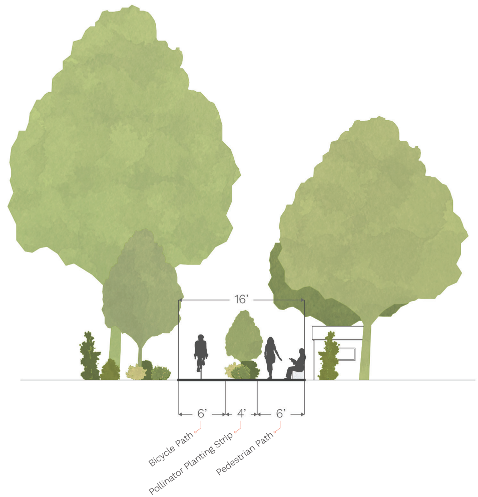
Figure 4.17: Auburn PL E Design Proposal Section
