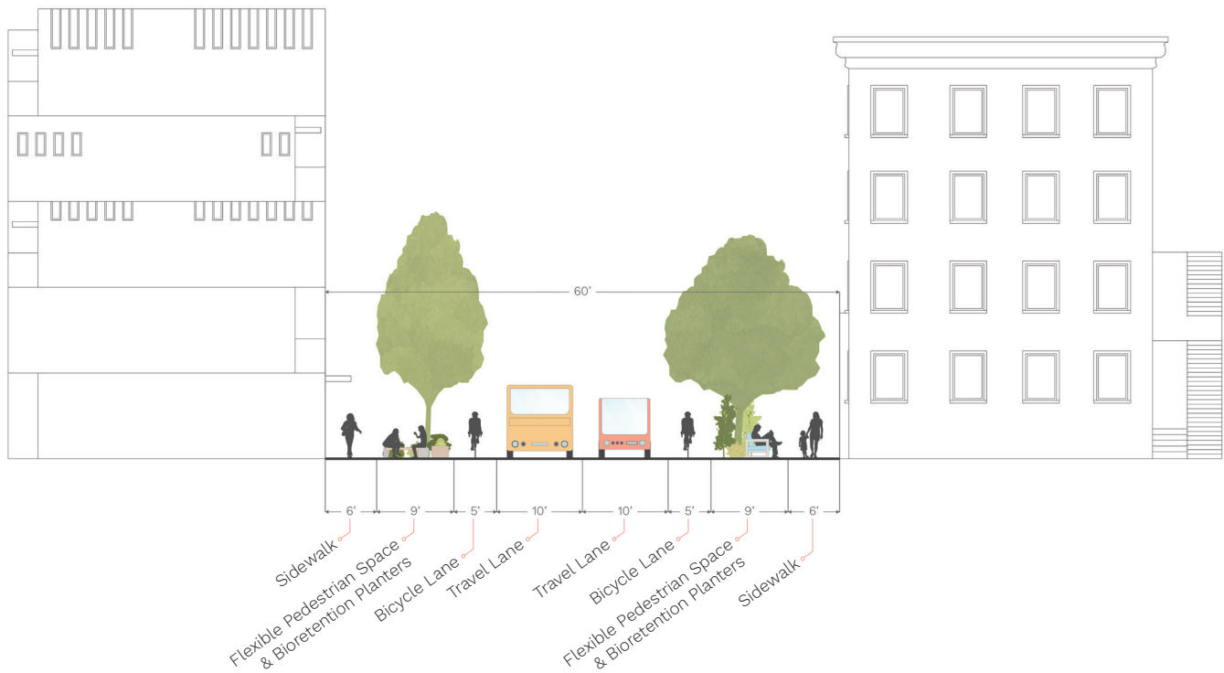
Figure 4.32: 10th Ave E Design Proposal Section (Facing North)
