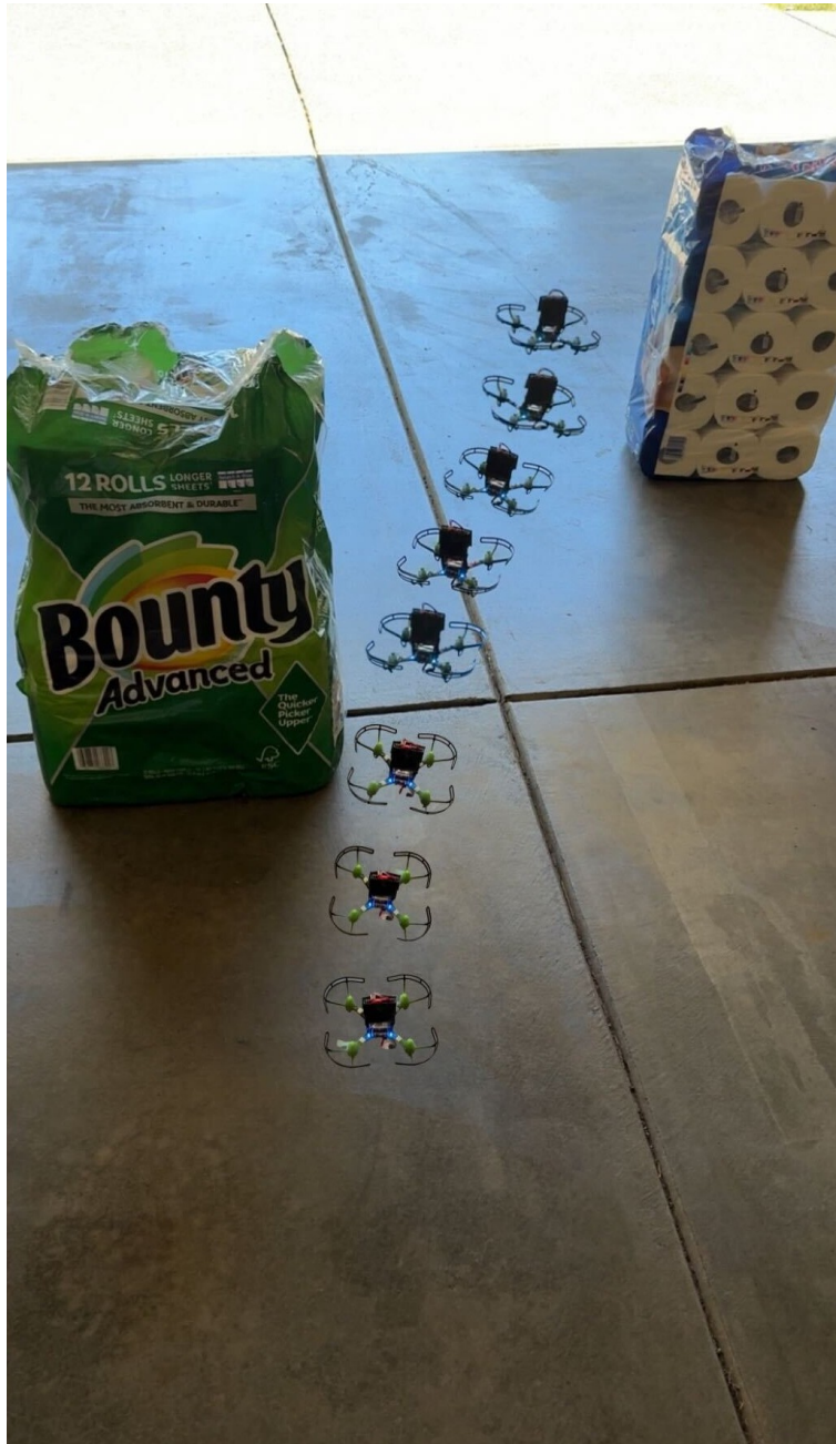
Figure 5.8: Obstacle avoidance using the onboard GenX320 event-camera module.
