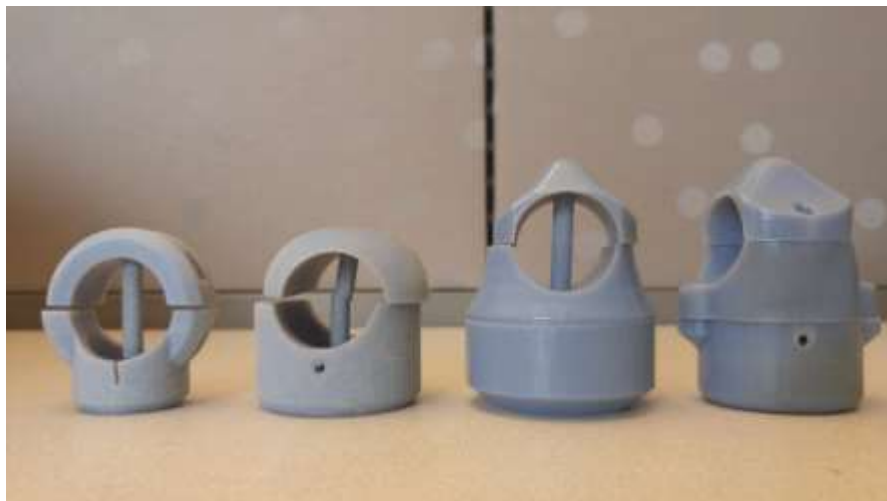
Figure 2.11: Iterative progression of housing design. Revisions increase from left to right.
