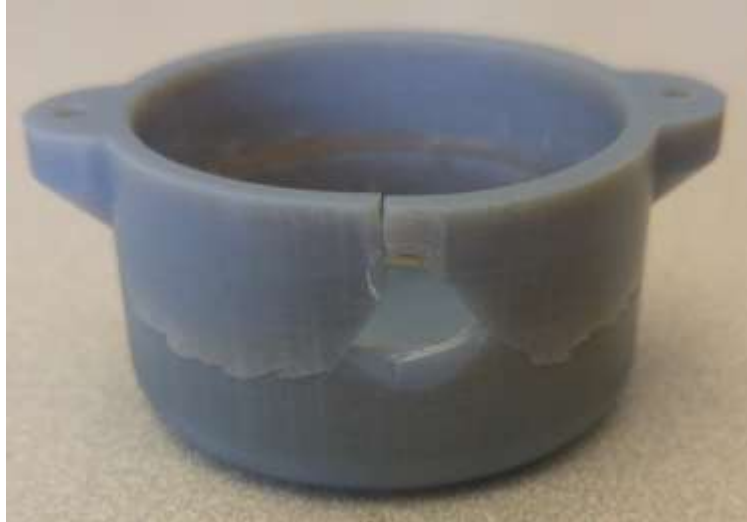
Figure 4.1: Fatigue failure of housing due to weak 3D printer material.
