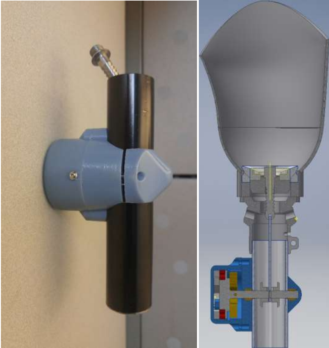
Figure 2.12: Left: RTP fully assembled on pylon stock. Right: Cross-section render of fully assembled system with socket and shuttle lock.
