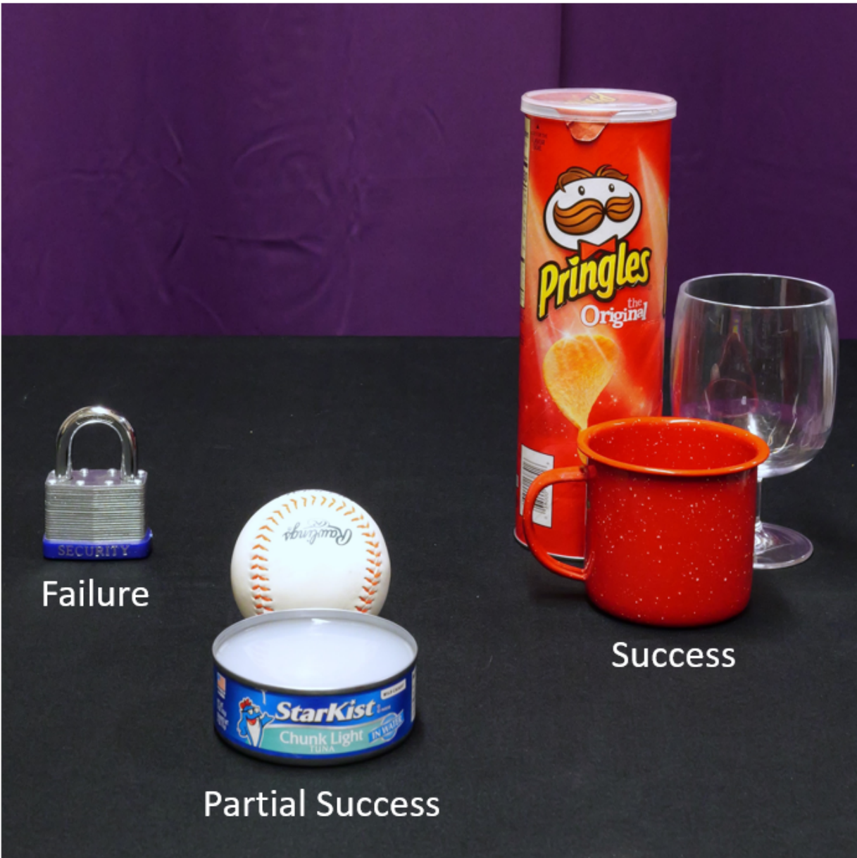
Figure 4.10: This figure shows the YCB objects we evaluated the TR-SLL gripper against. All of the items were chosen to be above the maximum demonstrated capacity for the Pneu-net gripper so any objects grasped show added capability. Additionally we filtered to non-box objects that fit within the jaws of the TR-SLL gripper. Of these items, the TR-SLL lifted five items successfully, with two being partial successes. The only failure is the padlock.
