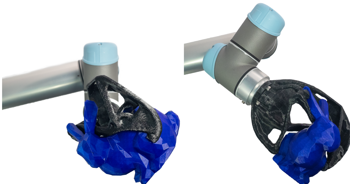
Figure A.10: Post-grasp stability test for the bunny. We measure the maximum roll angle both CW and CCW (left) and forward tilt angle (right) before the bunny falls.
