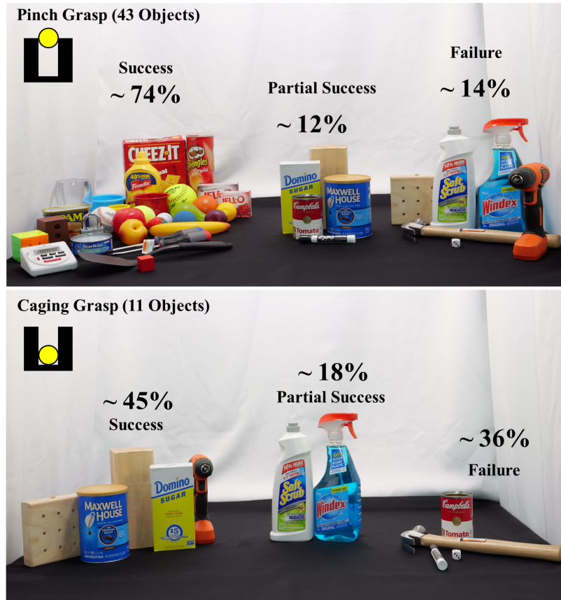
Figure 5.9: This figure shows the YCB test objects we evaluated the HSA gripper against. Objects were filtered to have a critical dimension that fit within the jaws of the gripper. First a pinch grasp was performed on the dataset. A success was defined as lifting the object and holding it for 30 seconds. A partial success was fulfilled if the object was able to be picked up but was not stable after 30 seconds. If the object was unable to be lifted off the ground, it was a failure. Of the objects that were not fully stable after the time period, a caging grasp was employed. The same success metrics were employed. The gripper was successfully able to lift all objects across both grasp modes. However, three objects only achieved a peak of partial success.
