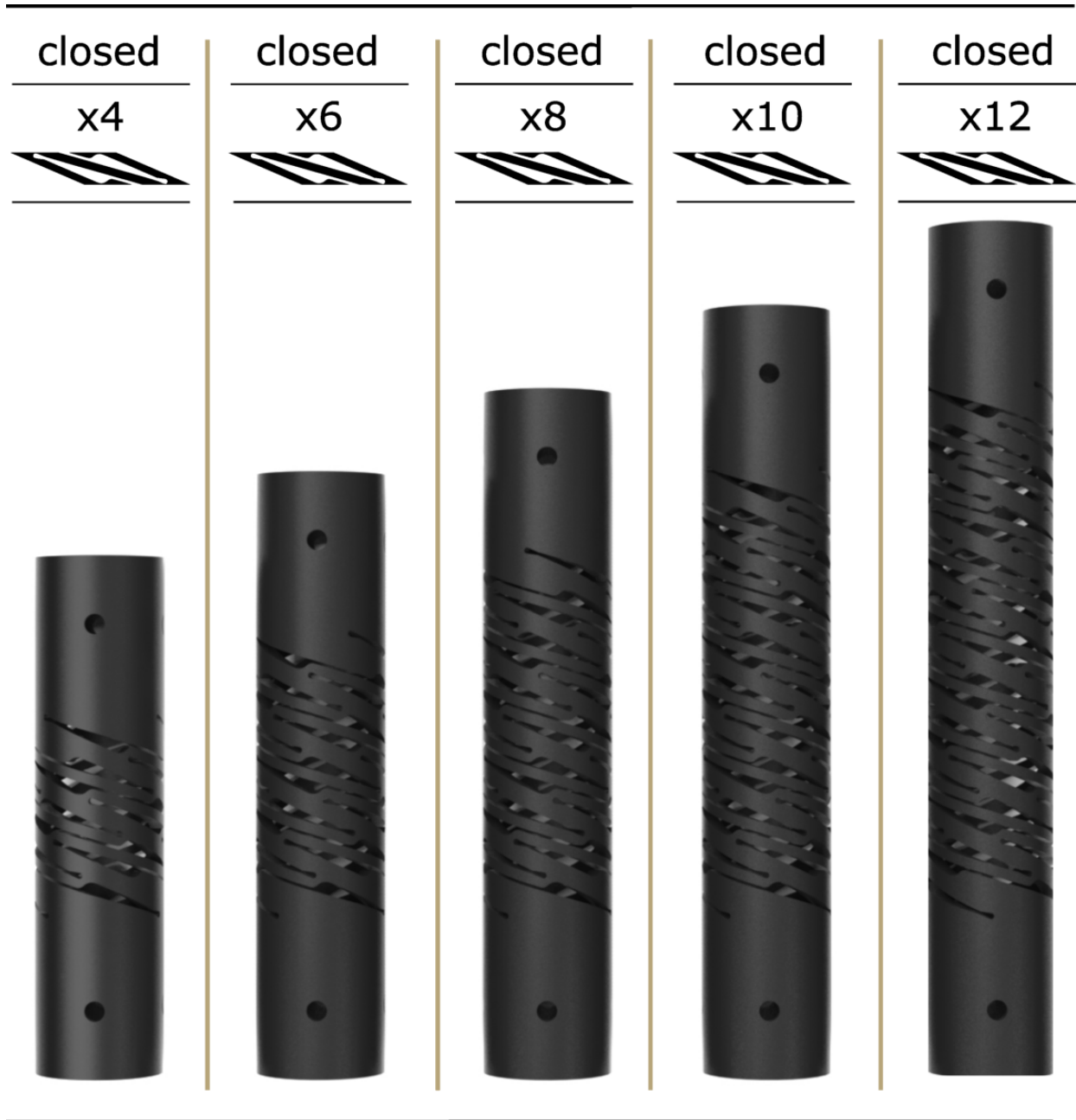
Figure 2.3: Five instantiations of closed left-handed HSAs with varying row tilings from four to twelve. These are made by vertically stacking the closed pattern around a unit cell.
