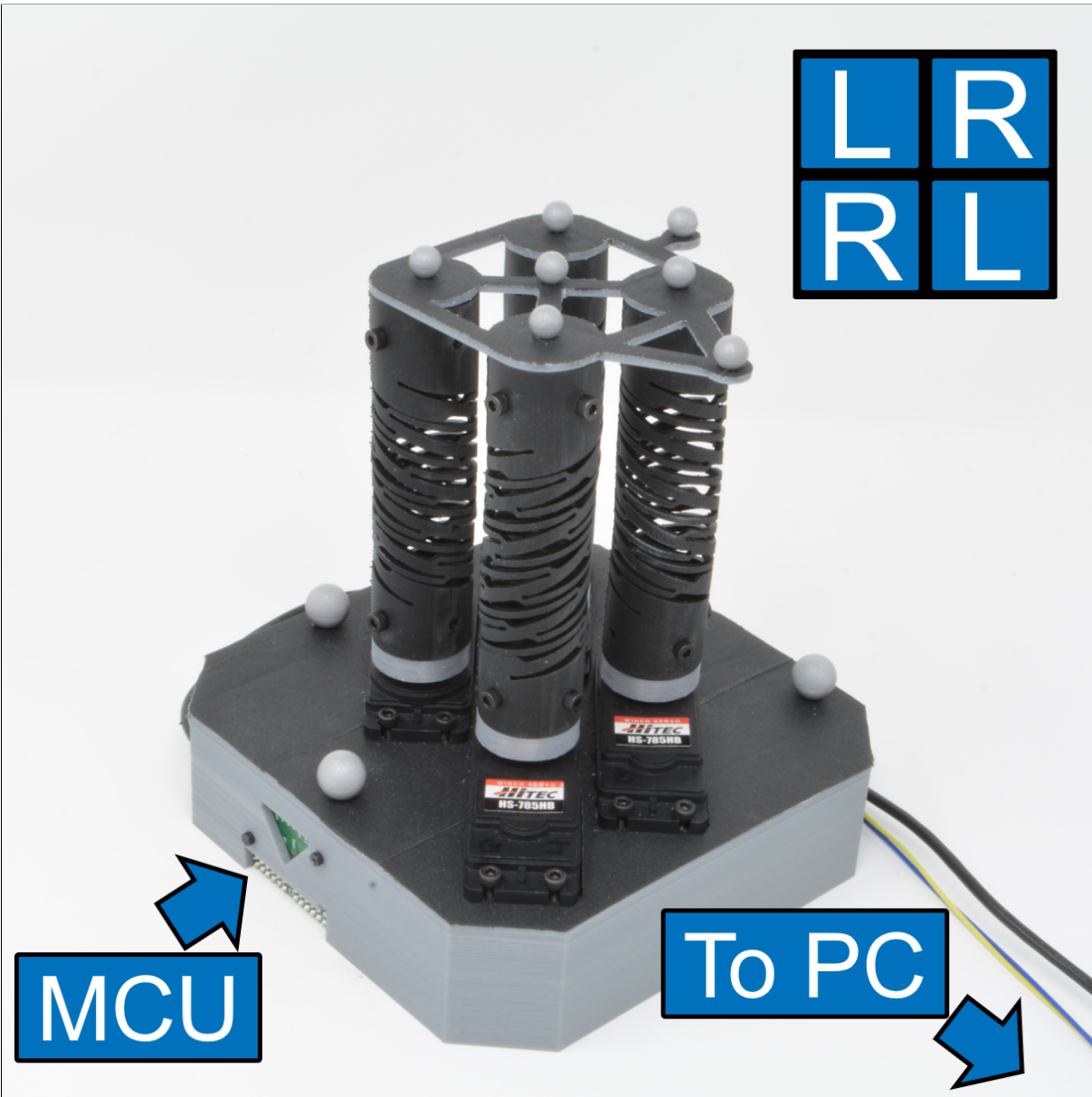
Figure B.6: The 2x2 HSA test platform. The top figure indicates the handedness of each HSA in the platform.
