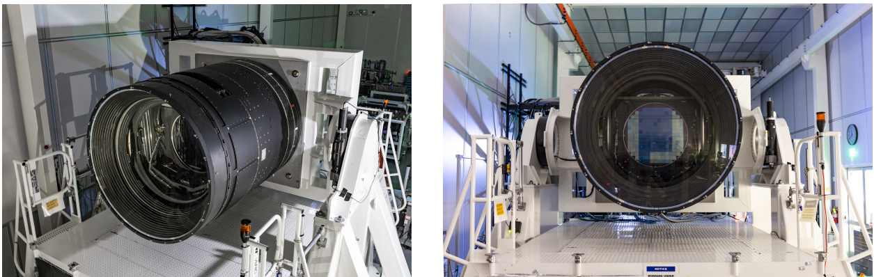
Figure 1.5: LSSTCam, the camera which will be used to conduct LSST. On the right you can see the focal plane of the camera, reflected in blue. The two different colors correspond to CCDs supplied by two different manufacturers. Image credit: Jacqueline Ramseyer Orrell/SLAC National Accelerator Laboratory.
