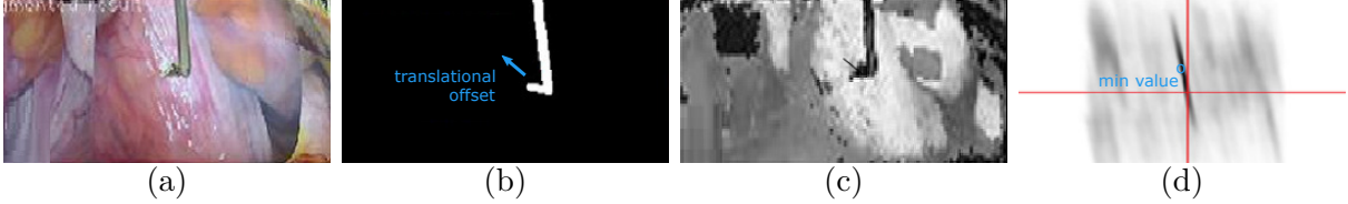
Figure 2.3: Translation matching. (a) raw image frame (b) initial shape prior mask, u (c) color filtering mask, Q (d) two masks convolved, minimum value gives optimal translational offset to generate mask U .
