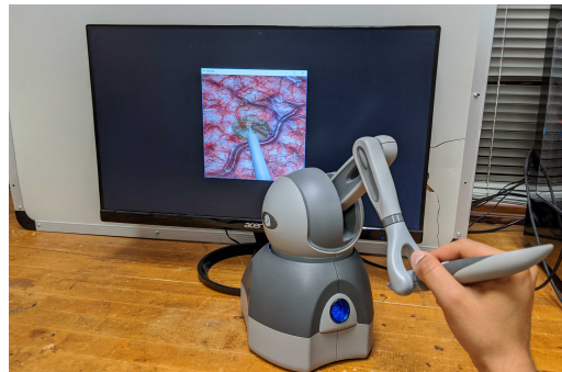
Figure 1.9: The experimental setup in [42]. Motion commands are sent and a deviated force feedback is received.
