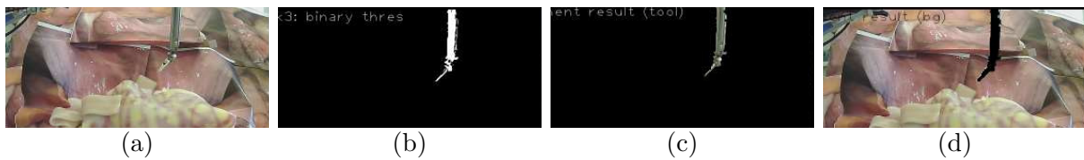
Figure 2.8: Raven II tool segmentation. (a) raw image (b) final shape prior mask (c) segmented foreground tool (d) segmented background tissue.
