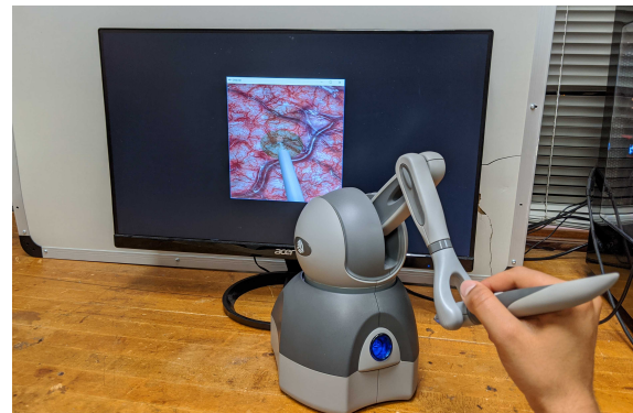
Figure 6.11: The experimental setup in [42]. Motion commands are sent and a deviated force feedback is received.
