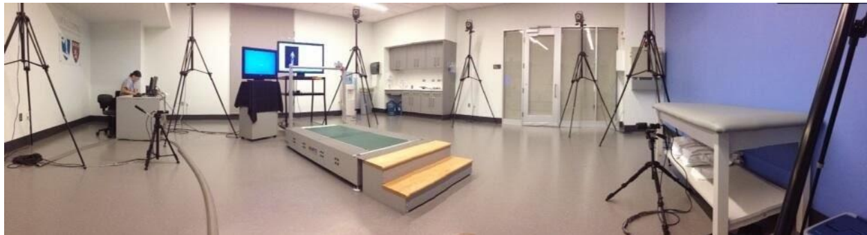
Figure 2.4: Gait analysis laboratory with an optical measurement system. Image taken from: http://runblogger.com/2013/10/my-running-gait-analysis-at-spaulding.html
