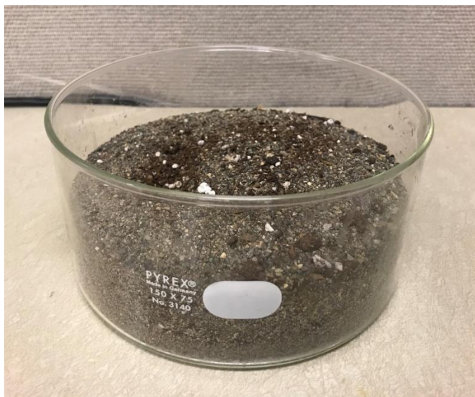
Figure 11: soil-sand mixture in the Pyrex® 150x75 mm crystallizing dish.
