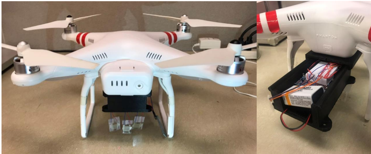
Figure 5: Drone set up for the drone test. Left: front view. Right: the 3D printed case for the battery and the Arduino board.
