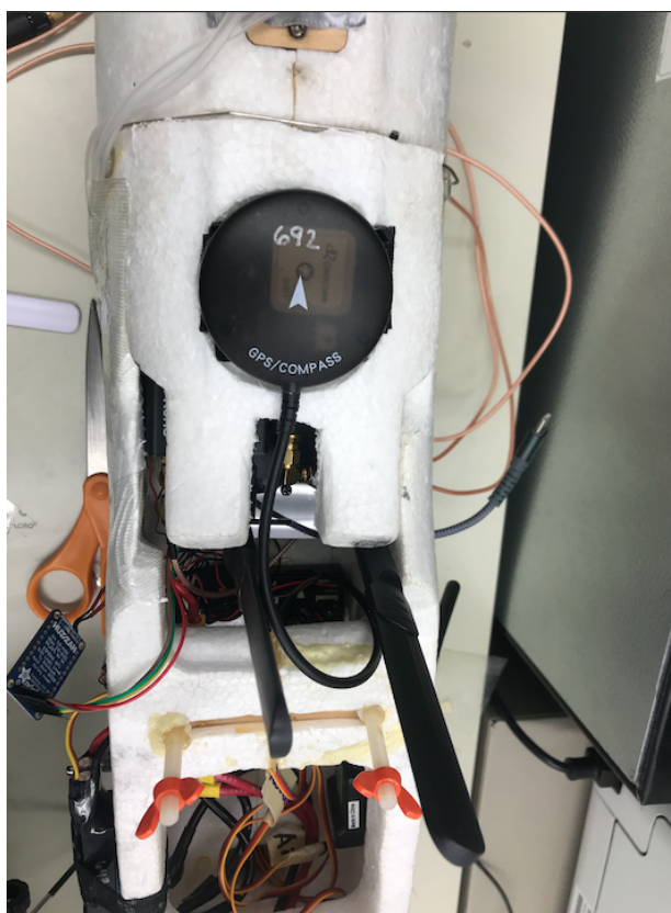
Figure 2.2: Top down view of closed aircraft payload bay containing WiCeNav payload. Note that the WiFi scraper remains fully inside the aircraft during flight, with only the antennas protruding, unlike this image.
