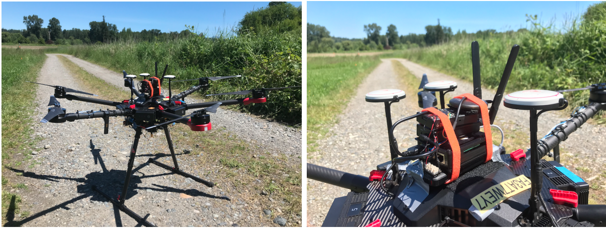
Figure 5.3: The DJI Matrice 600 Pro, nicknamed Aragog, with the CellNav payload (close-up at right) installed.
