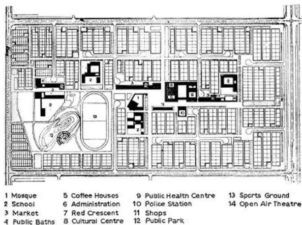
Figure 3: Plan of Community Sector in West Baghdad (Constantinos A. Doxiadis Archives, Human sector in Western Baghdad, Slides/9332)
