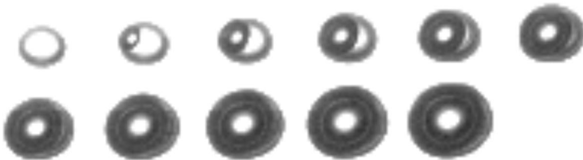
Fig. 3.7 – Stable homogenous boiling in a diethyl ether droplet of diameter, D_0 = 1.88 mm, immersed in glycerol at 5 bar pressure. Time between each image, \Delta t = 1 ms.
