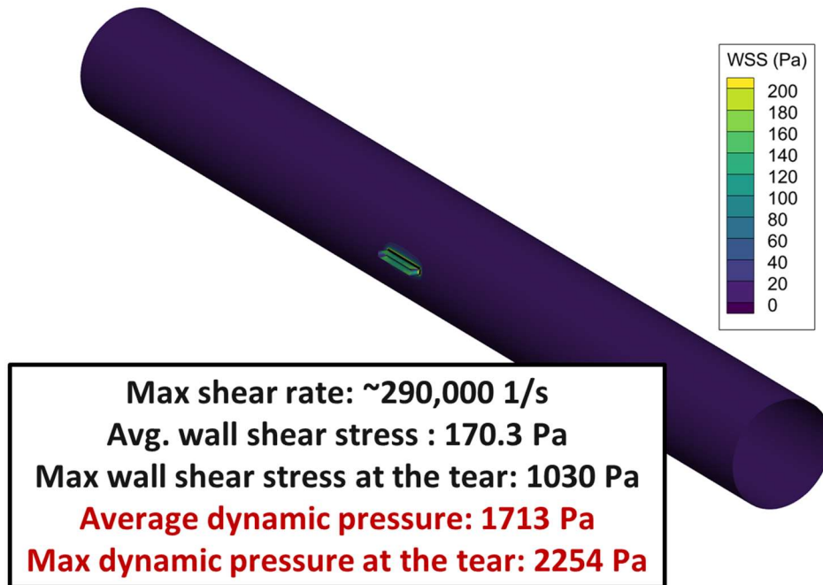
Figure 55. Simple pipe flow simulation of hemorrhage through a tear.
