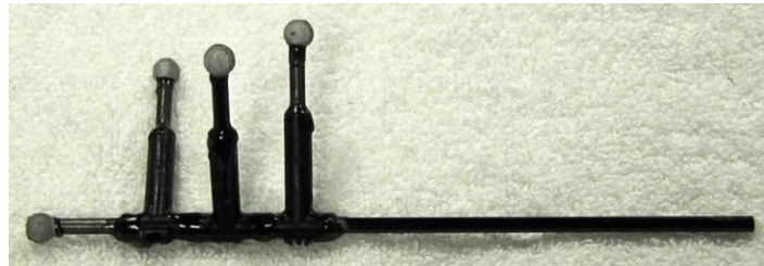
Figure 4.3: Vicon stylus used to digitize the CT bead fiducial markers. The tip of the stylus was machined to fit the spherical surface of the CT bead and calibrated to measure its center. The stylus used to digitize the orthopaedic bone screw fiducial markers had a pointed tip that fit into a small divot on the screw head.
