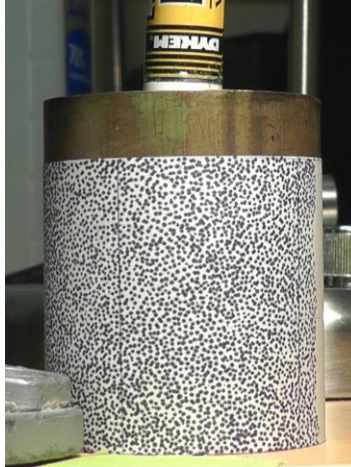
Figure 5.14: The specimen was placed on a flat surface and rotated about a spindle that passed through its center.
