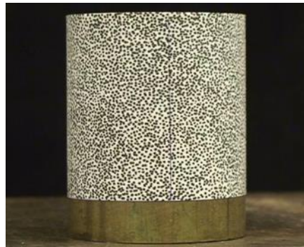
Figure 5.5: The specimen was a solid cylinder wrapped with a patterned piece of white paper.
