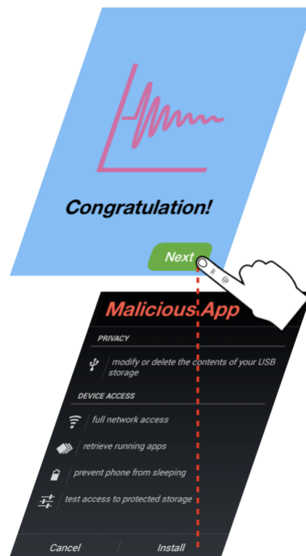
Figure 2.6. An example of "clickjacking". When user clicks the "next" button on the top-level overlay, the click event passes to the "install" button in the system dialog covered by the overlay.
