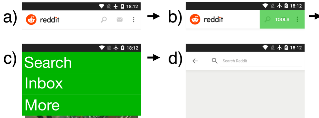
Figure 3.4. This interaction re-mapping replaces one interaction with a sequence of two interactions. (a) An interface contains small adjacent targets. (b) The targets are replaced with a single larger "Tools" button. (c) Selection displays a menu of the original targets. (d) A selected item is activated.
