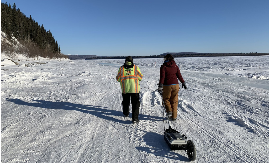
Figure 3.1 GPR measurements by Elizabeth Richards and Stan Zuray, Yukon River, February 27, 2020
