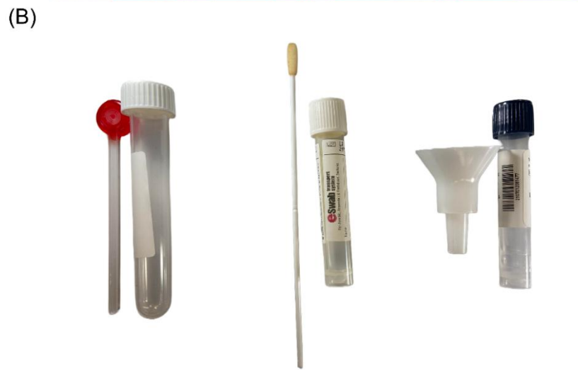
Figure B5. At-home saliva sampling devices for human subjects study. Self-saliva collection methods enable at-home sampling then shipping back to lab analysis. Three different collection methods included six CandyCollect devices, six ESwab™, and two SpeciMAX Stabilized Saliva Collection Kits (from left to right). (A) wrapped (B) unwrapped.
