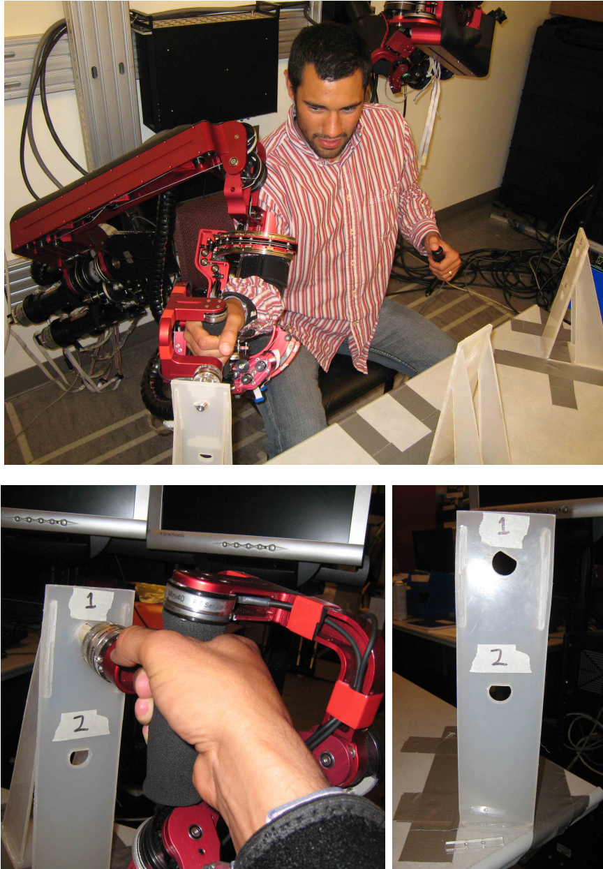
Figure 4.2: A subject inserts the tip of the exoskeleton into a target. There was a total of 6 targets. Each subject performed 4 repetitions of every controller moving to every target
