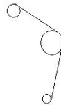
Figure 3.1: Each cable begins at the capstan, runs through intermediate pulleys and ends at a reduction pulley
