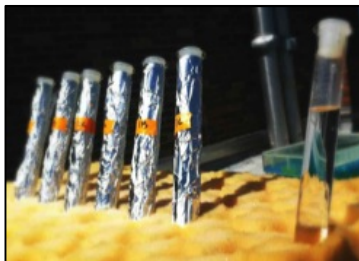
Figure 2.4: Outdoor quartz tube reactor set-up showing wrapped (left) and un-wrapped (right) tubes angled at approximately 60 degrees toward the sun.
